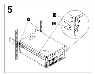
Fully extend the slide rails out of the rack. Lift the server above the rails; then, rest the racksupport wheels A located on the rear of the server on the slide rails. Lower the front of the server onto the slide rails.
