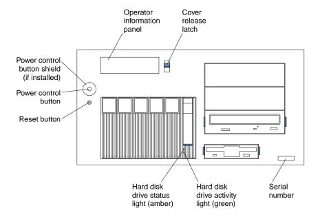
Power control button: Press this button to manually turn the server on or off.
