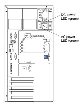
**AC power light:** This green light provides status information about the power supply. During normal operation, both the AC and DC Power lights are on. For any other combination of lights, see "Power supply LEDs" on page 146.
