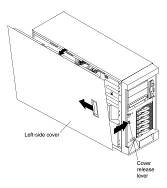
To remove the left-side cover of the tower model:
