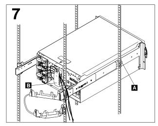
Press in on the safety latches **A** and slide the server halfway into the rack. Attach the power, keyboard, mouse, and monitor cables (if required) to the server and route them through the cable restraint bracket **B**. Then, attach all other required cables to the server.
