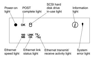
**Power-on light:** This green LED lights when system power is present in the server. When this light flashes, the server is in standby mode (the system power supply is turned off and current is present). If this light is not on, the power cord is not connected, the power supply has failed, or this LED has failed.
