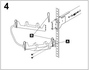
Use the M6 screws to attach the hinge bracket A to the rear of the rack. Then, use the hinge pins **B** to attach the cable-management assembly to the rack and to the slide rail (right rear of rack shown here).
