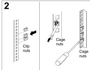
Slide on the clip nuts, or use a screwdriver or the cage-nut-insertion tool to insert the cage nuts, as required for your rack, into all the marked holes.
