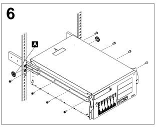
Use the M4 screws to secure the server to the rails. Remove the rack-support wheels A and store them in a safe place.
