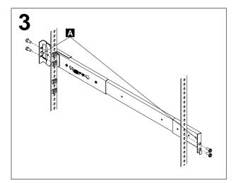
Use the pins **A** on the slide rail to align the slide rail to the rack. Use the M6 screws to bolt the slide rail to the rack (left front of rack shown here). Repeat this step for the other slide rail.
