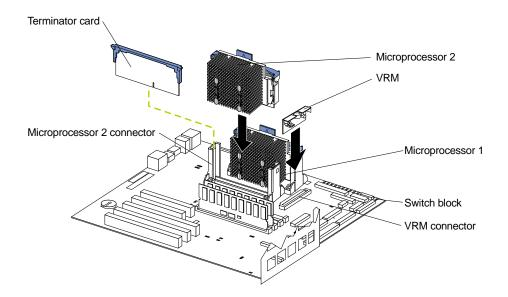
To install an additional microprocessor:
