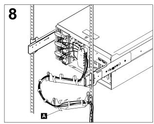
Route all the cables through the cablemanagement assembly as shown. Then, use the cable straps A or the cable ties to secure the cables to the cable-management assembly.
