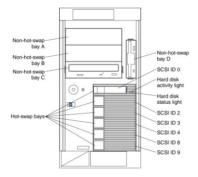
The SCSI IDs for the slim-high and half-high hot-swap drives are on a label Note: on the bezel, immediately adjacent to the hot-swap drive bays.
