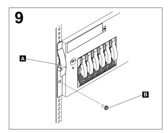
Slide the server into the rack until the release latches A snap shut. Then, insert the M6 screws **B** through the release-latch-bracket assembly. Note: Inserting the M6 screws B is optional, unless you are moving the rack or the rack is in a vibration-prone area.
