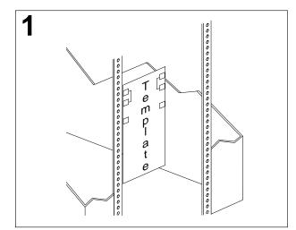
Use the attached stickers to mark the holes on the front and the rear of the rack in the locations indicated by the arrows on the template.
