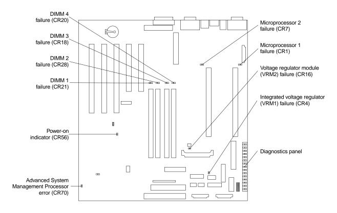
**Note:** The power-on indicator (CR56) lights when system power is present in the server. When this light flashes, the server is in standby mode (the system power supply is turned off and current is present).
